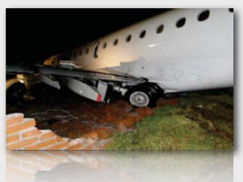
Ecuador's Junta Investigadora de Accidentes says the pilots attempted five times to reset the flaps, but that the slats would not deploy and the flaps would only move to position 2.
